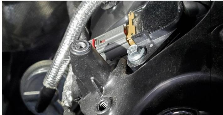
Use supplied screws to mount the bracket onto the Oil Separator, align logos so they match the same direction.
